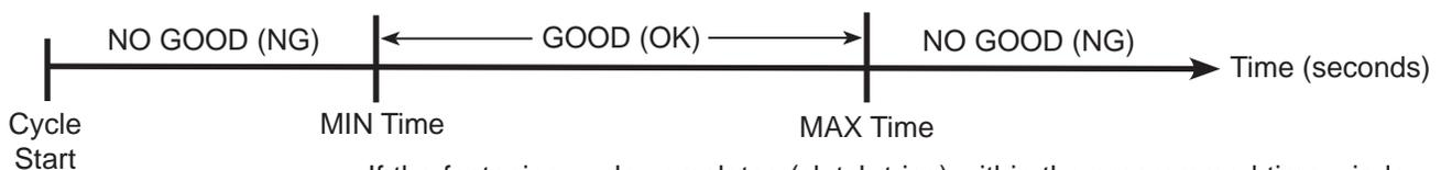
If the fastening cycle completes (clutch trips) within the programmed time window, the rundown cycle will be accepted as GOOD (OK) and the batch count will increment.
